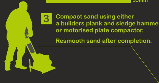
**3** Compact sand using either a builders plank and sledge hammer or motorised plate compactor.
