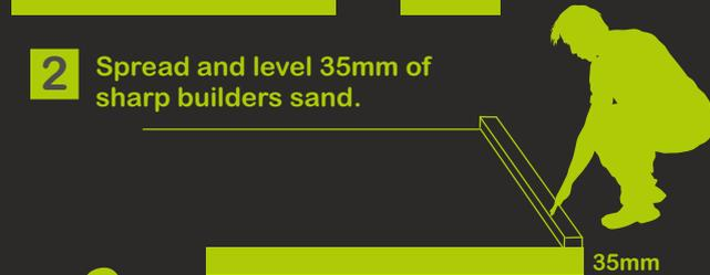
**2** Spread and level 35mm of sharp builders sand.
