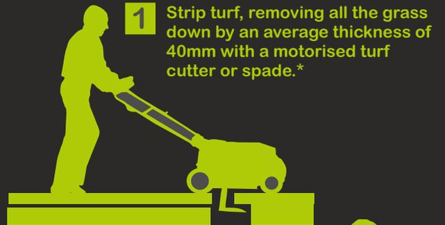
**1** Strip turf, removing all the grass down by an average thickness of 40mm with a motorised turf cutter or spade.\*
