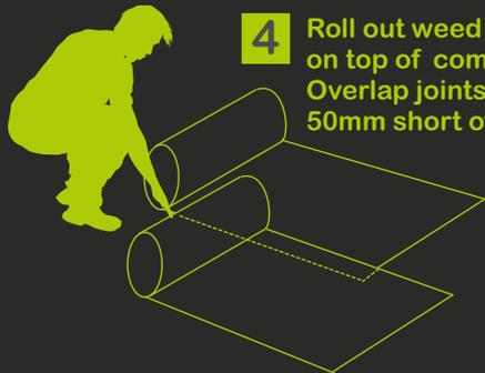
**4** Roll out weed retaining membrane on top of compacting sand. Overlap joints by 300mm leaving 50mm short of the grass edge.
